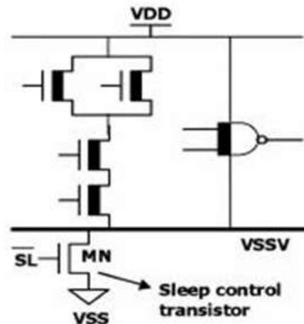
Figure 6 Schematic of Sleep Transistor circuit
