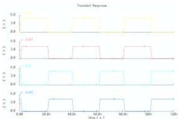
Figure 9 Transient Response of the bulk SRAM Cell
