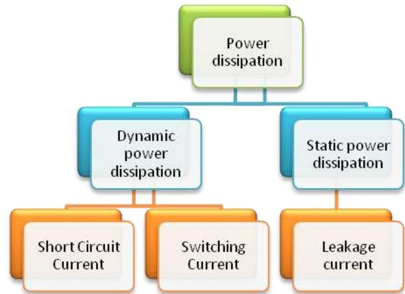
Figure 3 Hierarchy of the Power Dissipation
