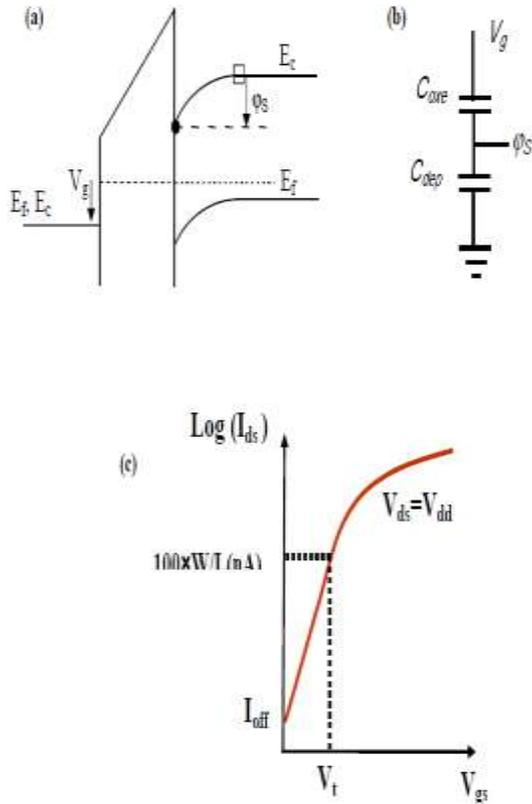
Figure 5: (a) When  $V_g$  is increased,  $E_c$  at the surface is pulled closer to  $E_f$ , causing  $n_s$  and  $I_{ds}$  to rise; (b) equivalent capacitance network; (c) Subthreshold IV with  $V_t$  and  $I_{off}$
