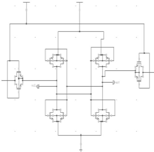
Figure 2 DG-MOSFET based 6T SRAM Cell
