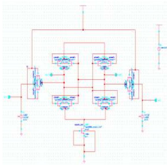
Figure 14 Circuit of the DG-MOSFET Based 6T SRAM Cell with sleep transistor
