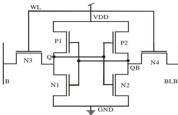
Figure 1 Conventional 6T SRAM Cell
