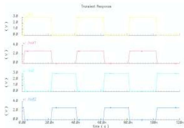
Figure 10 Transient Response of the Proposed DG-MOSFET Based 6T SRAM Cell
